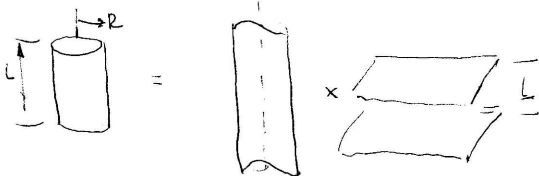
$$\left( \frac{T(t, x, r) - T_{\infty}}{T_i - T_{\infty}} \right) = \underbrace{\left( \frac{T(t, x) - T_{\infty}}{T_i - T_{\infty}} \right)}_{\text{short cyl}} \times \underbrace{\left( \frac{T(t, r) - T_{\infty}}{T_i - T_{\infty}} \right)}_{\text{oo long cyl}}$$
