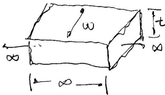
$$\left( \frac{T(t, x, y) - T_{\infty}}{T_i - T_{\infty}} \right) = \underbrace{\left( \frac{T(t, x) - T_{\infty}}{T_i - T_{\infty}} \right)}_{\text{along rectangl bar}} \times \underbrace{\left( \frac{T(t, y) - T_{\infty}}{T_i - T_{\infty}} \right)}_{\text{horiz || plates wall}}$$
